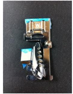
32. Set the stitch length to 3 for easier feeding. Lower the presser foot and take a few stitches. This will anchor the fabric. Now move the needle position to the left until it is close to the left edge of the fabric. Take a few more stitches to check the position and adjust as necessary.
