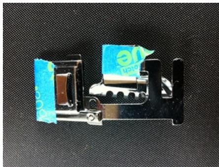
29. The foot has an adjusting screw on the top. Loosen the screw and move to the right side of the opening, shifting the whole foot to the left.
